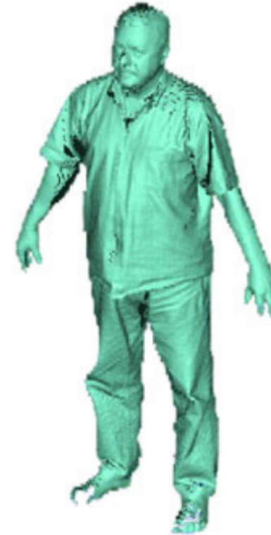
Fig. 7.9 Left: The (laser) light source projects a sweeping light plane (by fanning out a light beam into a “sheet of light”), which projects at each time a bright line across the objects of interest. Right: The recovered surface of a person using structured lighting
