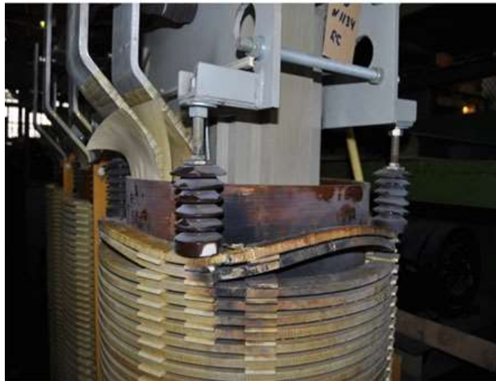
Fig. 1.16 Axial winding displacement
