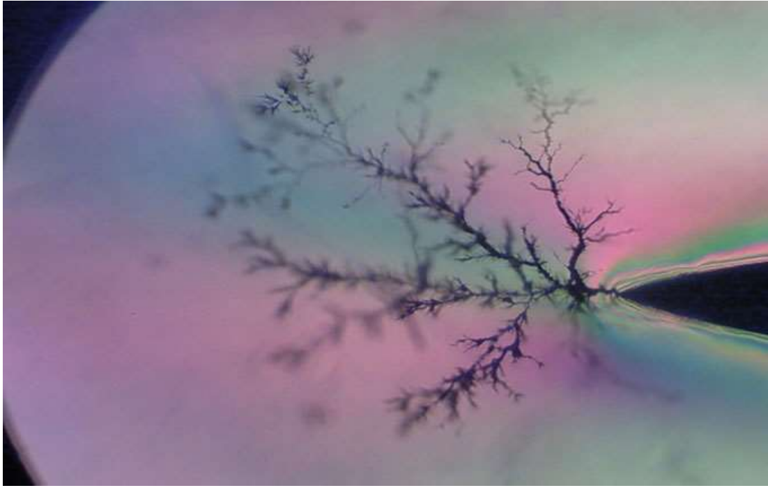
Fig. 1.9 Photo of a dendrite in a translucent polymer dielectric
