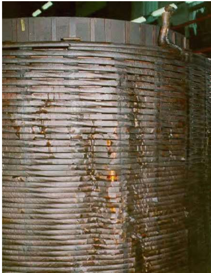
Fig. 1.13 Radial displacement of winding turns
