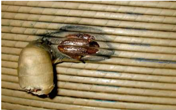
Fig. 1.18 “Short-circuited turn” type of winding defects
