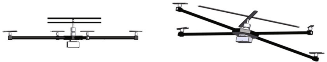
Fig. 1.4 A compound multicopter. The middle coaxial propellers with a slow dynamic response provides the main lift, while the surrounding quadcopter can change the propeller angular speeds rapidly to improve the dynamic response of attitude
