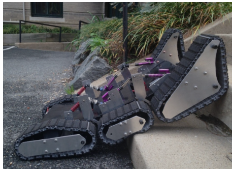
Ground Drone Project: Urban mobile robot chassis.
