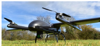
Hybrid Propulsion Fixed-Wing VTOL Drone.
