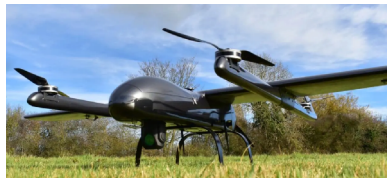
Hybrid Propulsion Fixed-Wing VTOL Drone.
