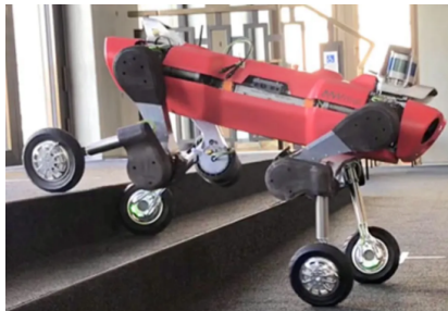
Quadruped robot ANYmal on wheels.
