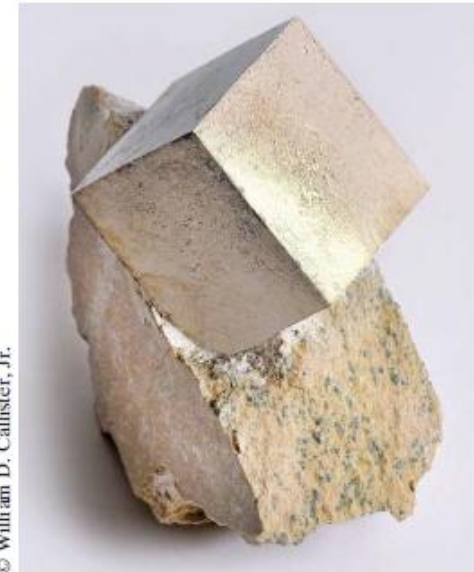
Figure 3.18 An iron pyrite single crystal that was found in Navajún, La Rioja, Spain.
