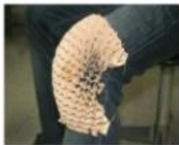
Knee-cap made up of auxetic network
