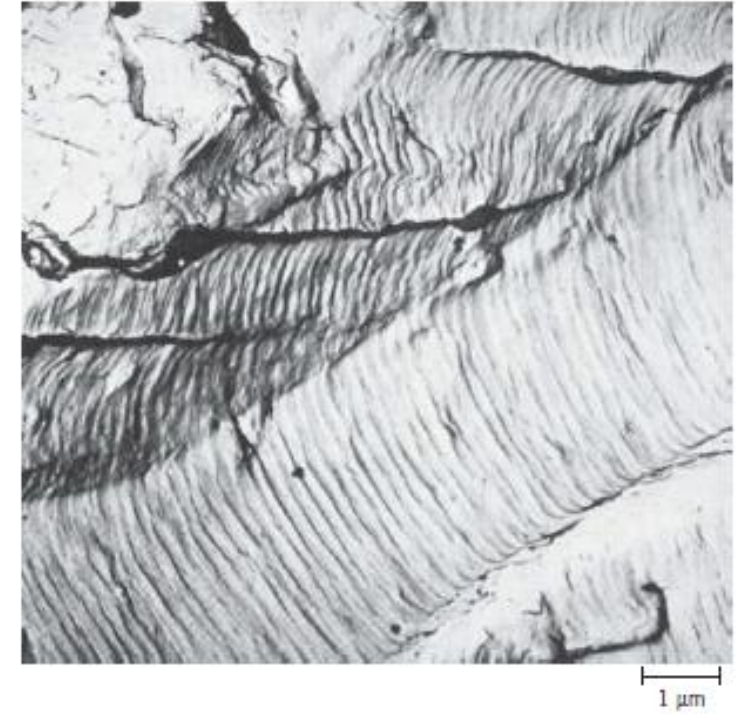
Figure 8.24 Transmission electron fractograph showing fatigue striations in aluminum. 9000 \times . (From V. J. Colangelo and F. A. Heiser, Analysis of Metallurgical Failures , 2nd edition. Copyright © 1987 by John Wiley & Sons, New York. Reprinted by permission of John Wiley & Sons, Inc.)
