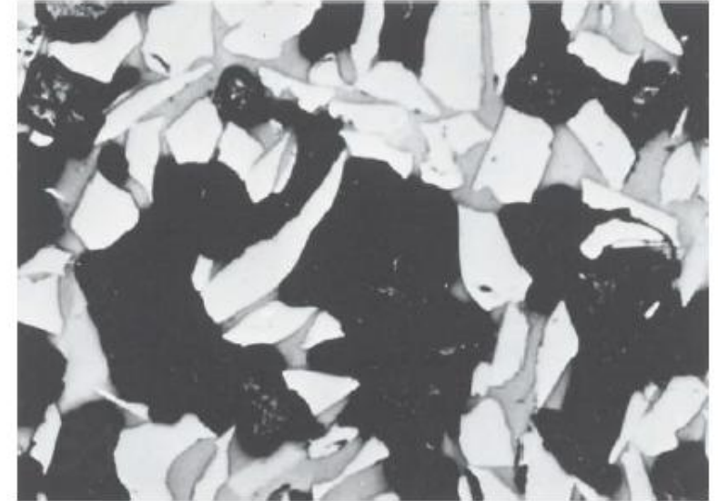
Figure 13.5 Photomicrograph of an aluminum oxide–bonded ceramic abrasive. The light regions are the \text{Al}_2\text{O}_3 abrasive grains; the gray and dark areas are the bonding phase and porosity, respectively. 100 \times . (From W. D. Kingery, H. K. Bowen, and D. R. Uhlmann, Introduction to Ceramics , 2nd edition, p. 568. Copyright © 1976 by John Wiley & Sons. Reprinted by permission of John Wiley & Sons, Inc.)
