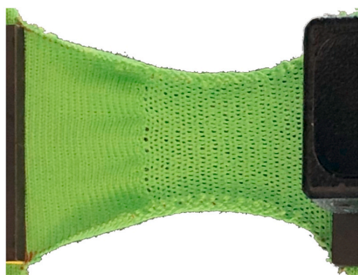
(a) A physical course-wise tensile test at 30% strain
