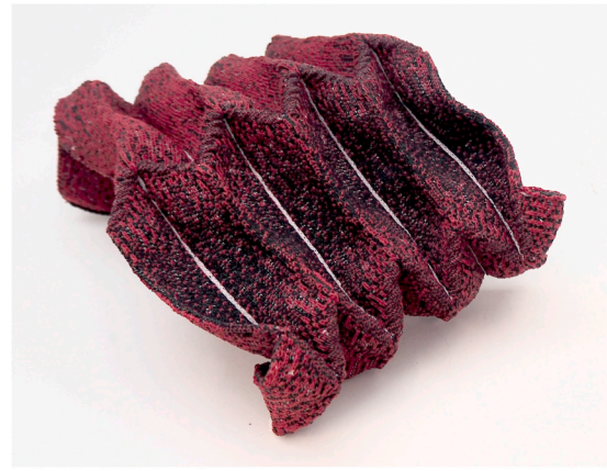
Fig. 1. Examples of knitted textiles with 3D shapes, graded stitch patterns and varying knitting directions.
