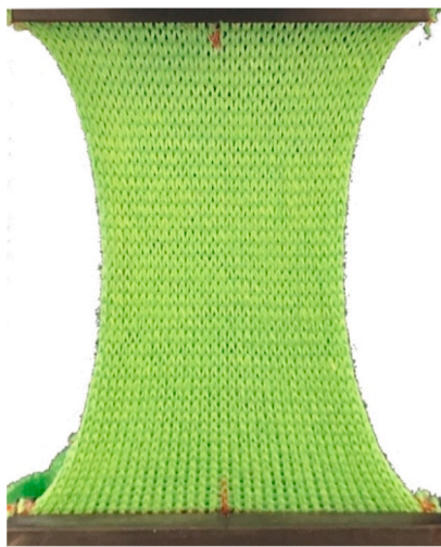
(c) A physical wale-wise tensile test at 30%
