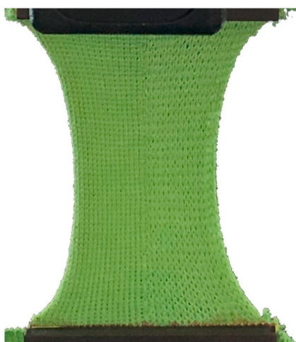
(c) A physical wale-wise tensile test at 30% strain
