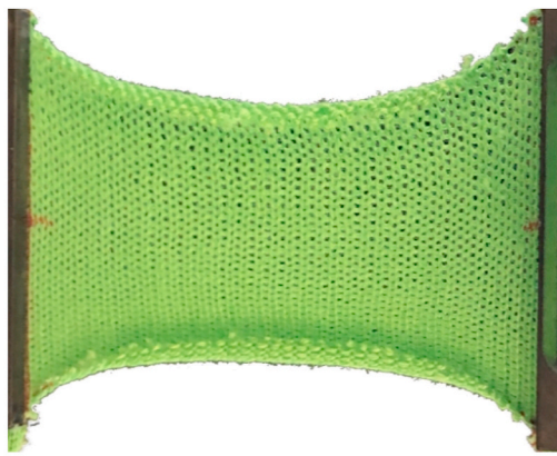
(a) A physical course-wise tensile test at 30% strain
