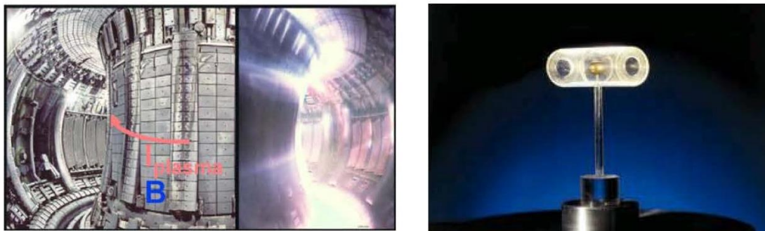
Figure 3: On the left: photograph of the interior of the JET tokamak chamber. On the right: photograph of the laser-irradiated target for inertial confinement fusion.
