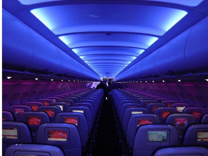
LED lighting in the aircraft cabin of an Airbus A320 Enhanced .
