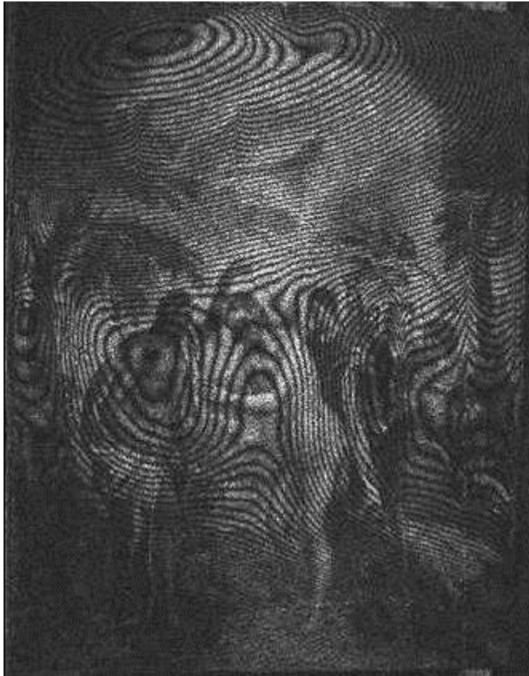
Interferogram indicating surface movement recorded after climate change (10% → 44% RH)
