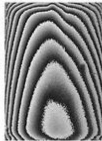
Interferogram indicating surface movement recorded after climate change (10% → 44% RH)
