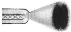
Output from a fibre supporting two modes
