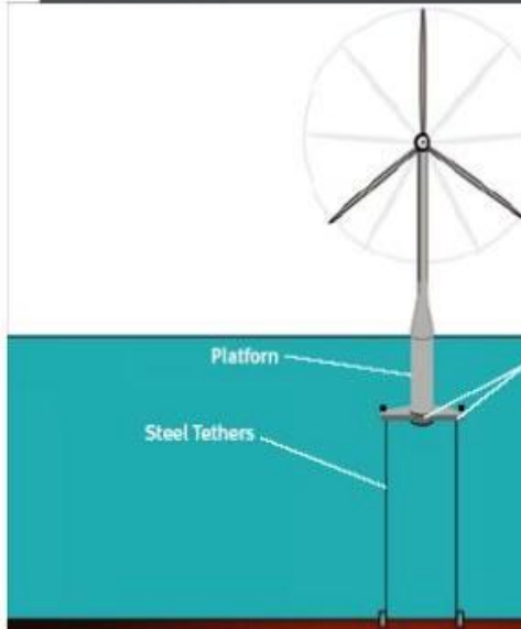
TENSION LEG PLATFORM FLOATER
