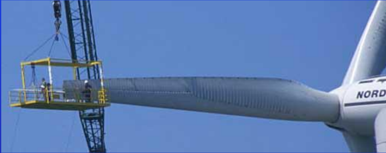
Tip vane extension on the rotor blade of the Enercon E-66 wind turbine
