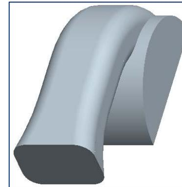
**Figure K** Default view of the model after creating a round feature of radius 1.5
