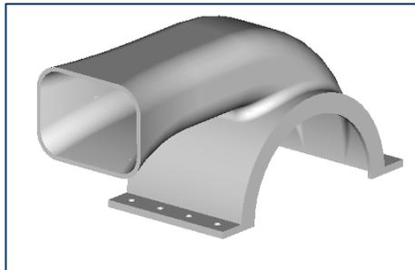
**Figure A** Solid model of the Upper Housing
