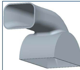
**Figure N** The model after shelling
