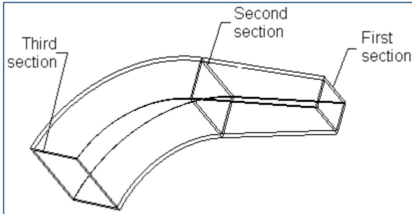
**Figure A** Three sections in swept blend
