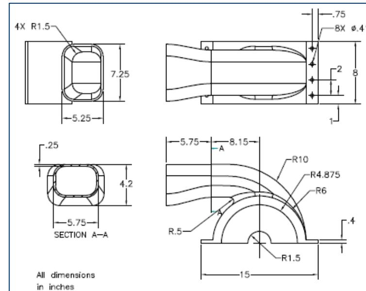
**Figure B** Left-side view of the top view, top view, front view, and the sectioned left-side view of the model
