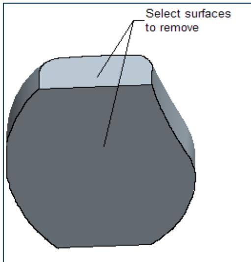
**Figure K** Surfaces to be selected to remove
