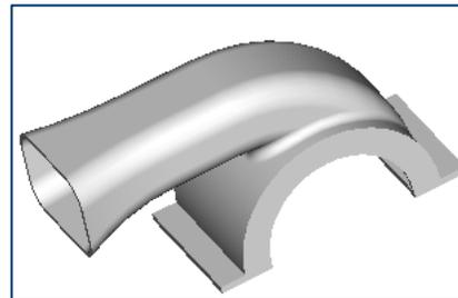
**Figure U** Model after mirroring the extrude feature
