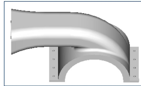
**Figure W** Hole patterned on the extruded features
