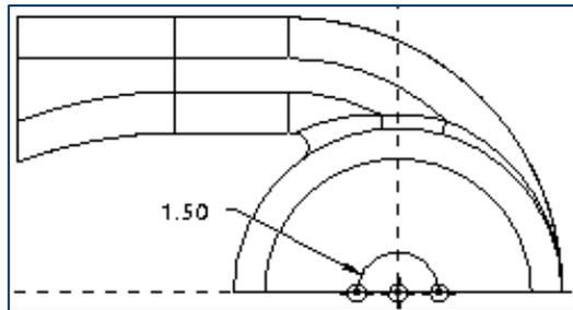
**Figure Q** Sketch with dimension for the cut feature
