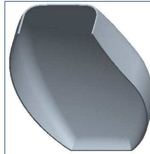
**Figure L** Final model after shelling
