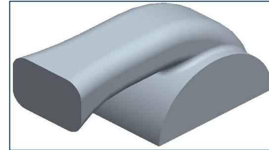
**Figure M** Model after creating a round feature of radius 0.5
