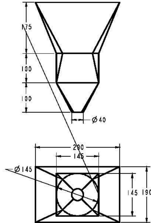
Figure 8-111 Top and front views of the model
