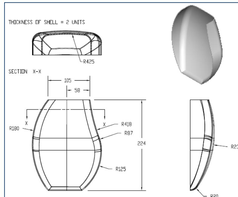
**Figure B** Sectioned-top, front, right- side, and isometric views of the model
