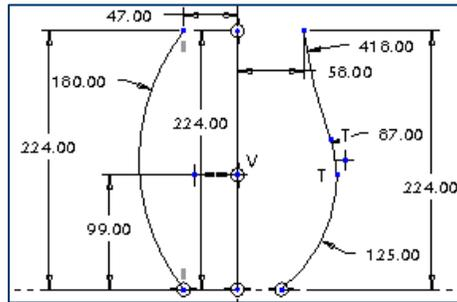
**Figure D** Sketch with dimension of the additional trajectory
