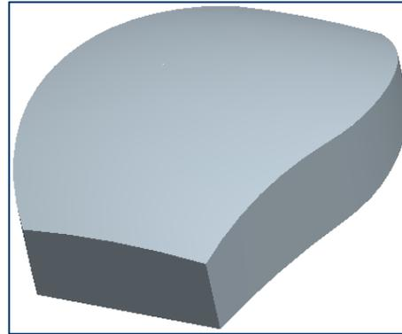
**Figure H** Variable section sweep feature
