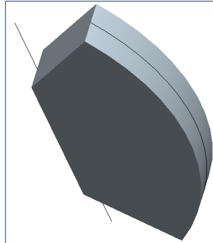
**Figure D** Resulting variable section sweep feature
