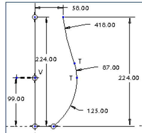
**Figure C** Sketch with dimensions of the X trajectory
