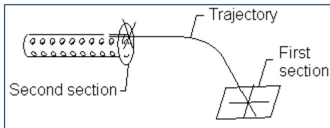
**Figure C** Two sections and a trajectory
