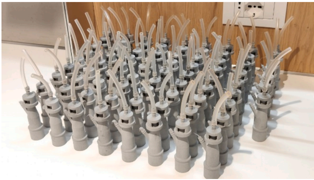
Fig. 4. Respiratory valves designed and printed in just 24 -hs [29].
