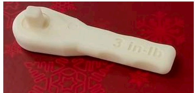
Fig. 3. Wrench printed in space on the International Space Station [28].
