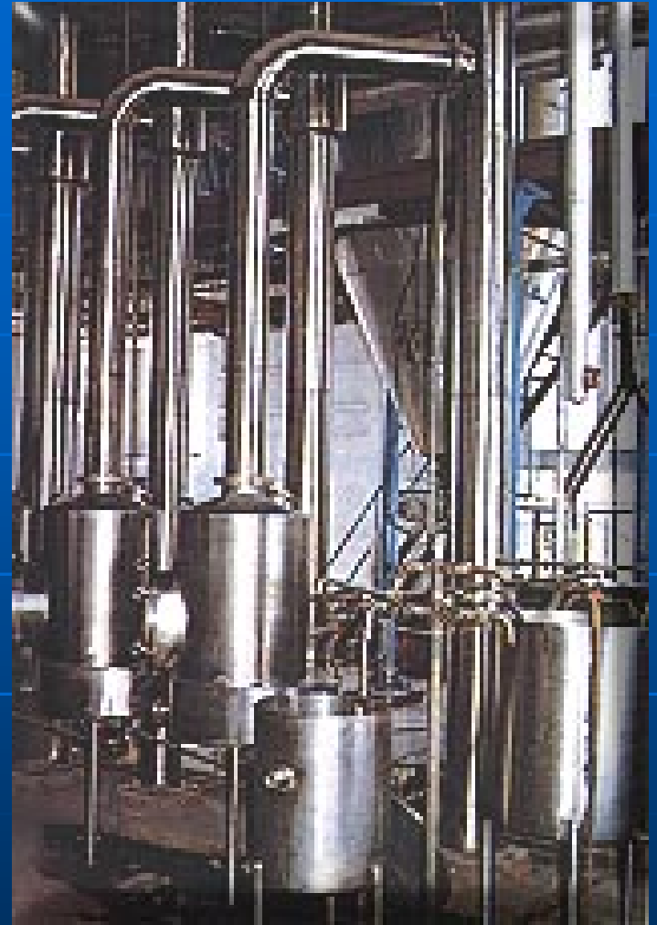
Falling film evaporator
