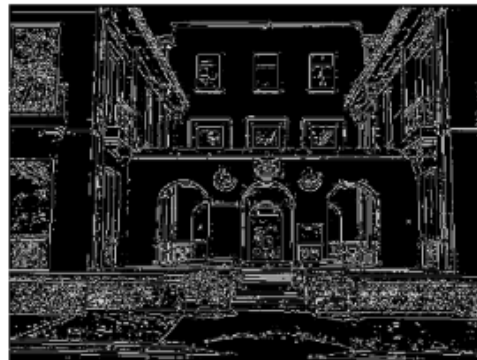
low threshold (weak edges)
