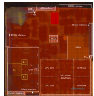
Apple A7, 28nm TSMC, 102mm 2
