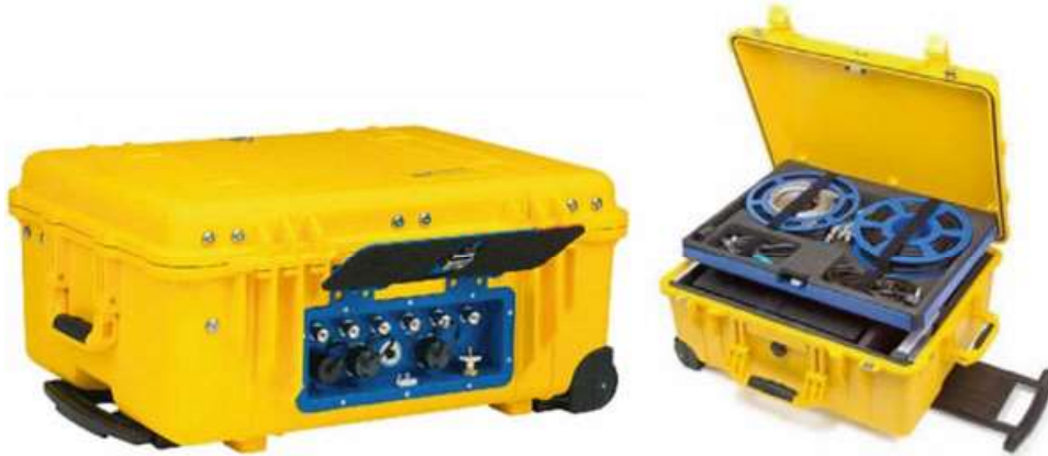
Fig. 2.8 Portable system for measuring and periodic monitoring of partial discharges in diverse high-voltage equipment, Omicron OMS-605
