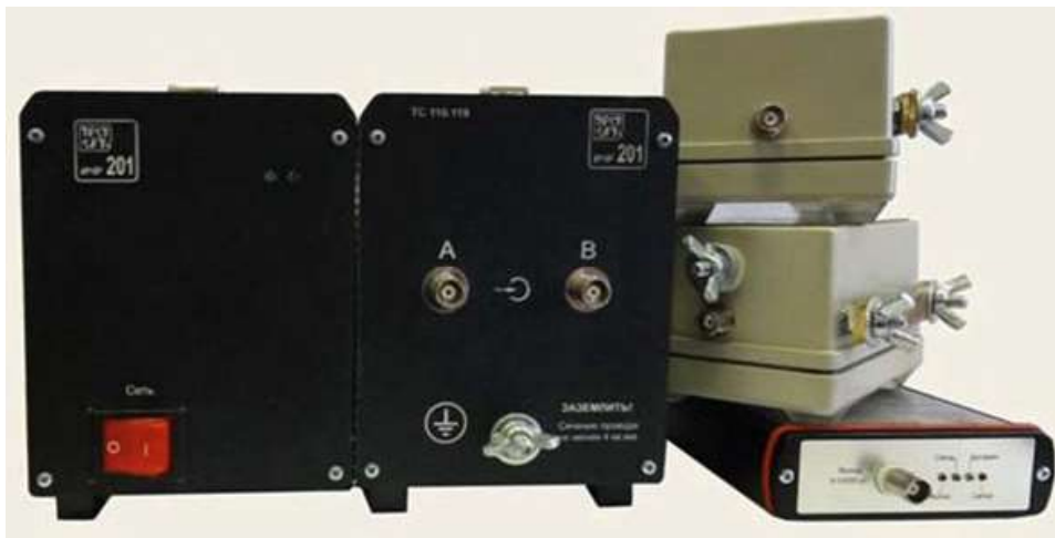
Fig. 2.13 Partial discharge indicator IChR 201
