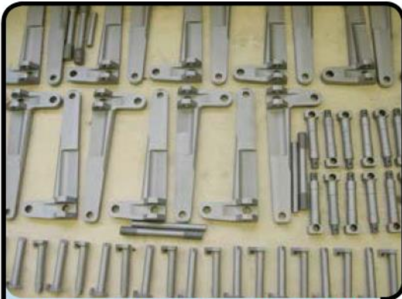
Levers and Pins: Chromium Carbide coating for wear resistance
