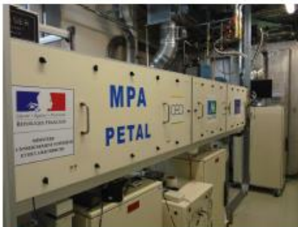
The pre-amplification module of PETAL
