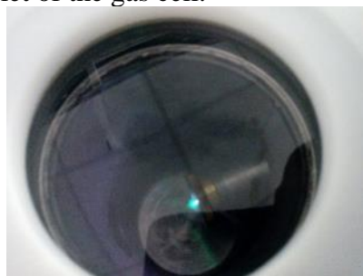
Figure 2.3 Gas cell. Is visible the plasma created by the focused beam on copper foil creating the outlet of gas cell.
