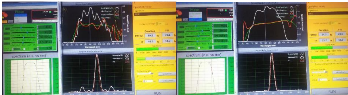
Figure 1.12: Pulse improvement by feedback to Dazzler. Before feedback (left) the best measurements results by changing the grating distance of the compressor or the polynomial parameters of Dazzler are far away from the calculated Fourier Transform Limited (FTL) and the phase spectrum is not flat enough. After few feedback steps to Dazzler (right) the phase spectrum is optimized and the measured pulse characteristics is near the ideal FTL.
