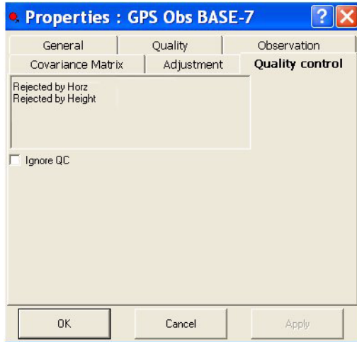
Figure B-21. Quality Control for GPS Observation that Fails TS Obs Precisions
