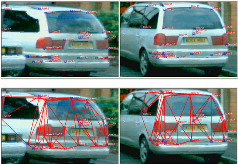
Figure 10-9. Creating Surface for Measured Points
